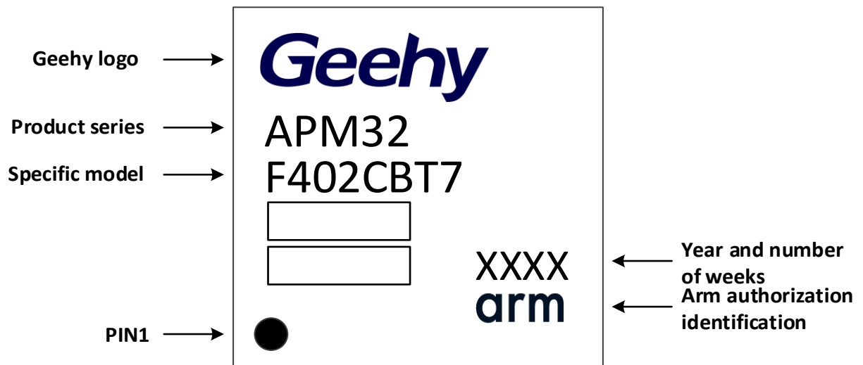
Figure 21 LQFP48 -48 Pins, 7x7mm Identification
