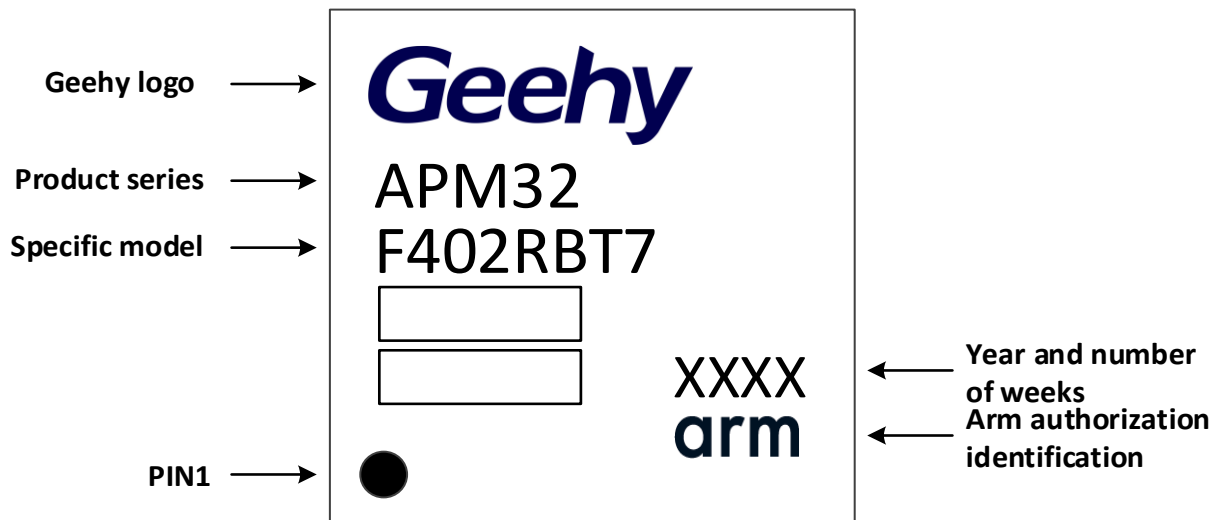
Figure 18 LQFP64 - 64 Pins, 10 x 10mm Package Identification
