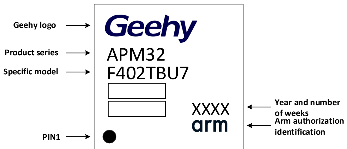
Figure 27 LQFN36-36 Pin 6x6mm Identification
